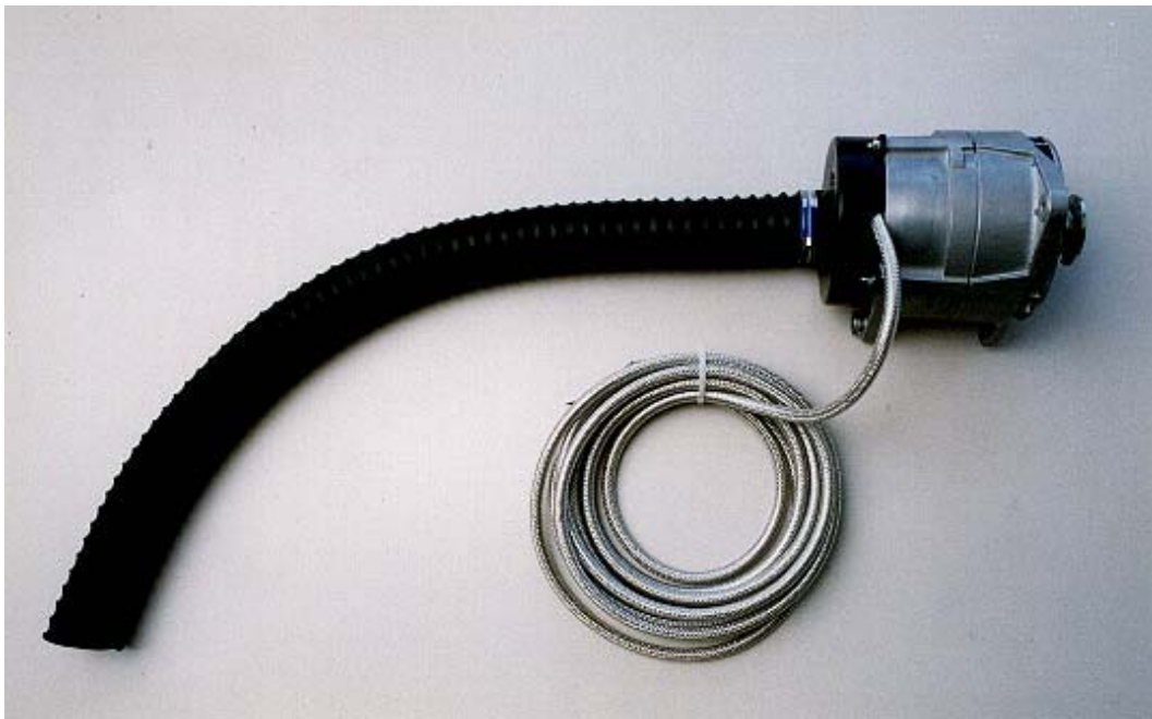
Generator with DIA 55mm air intake hose Cut any place at the rear cover for gen.cable exit
